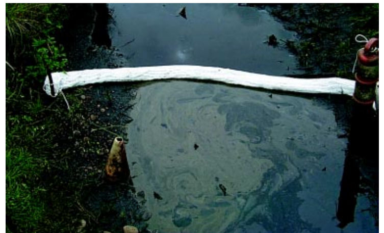
When oil spills into a local waterway, booms are used to contain it so it doesn't spread. The oil can then be soaked up with absorbent material.
