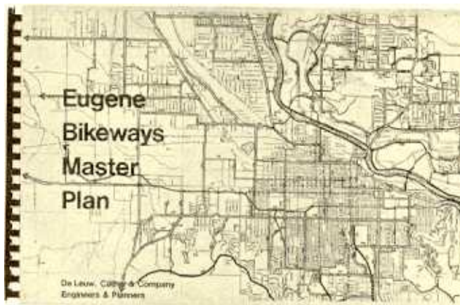
THE EUGENE BIKEWAYS MASTER PLAN , not a dusty document on a back shelf, gets regular use and yearly update. By the end of 1981, the bikeway network included 21 miles of independent paths, 34 miles of striped lanes, and 15 miles of signed routes.
